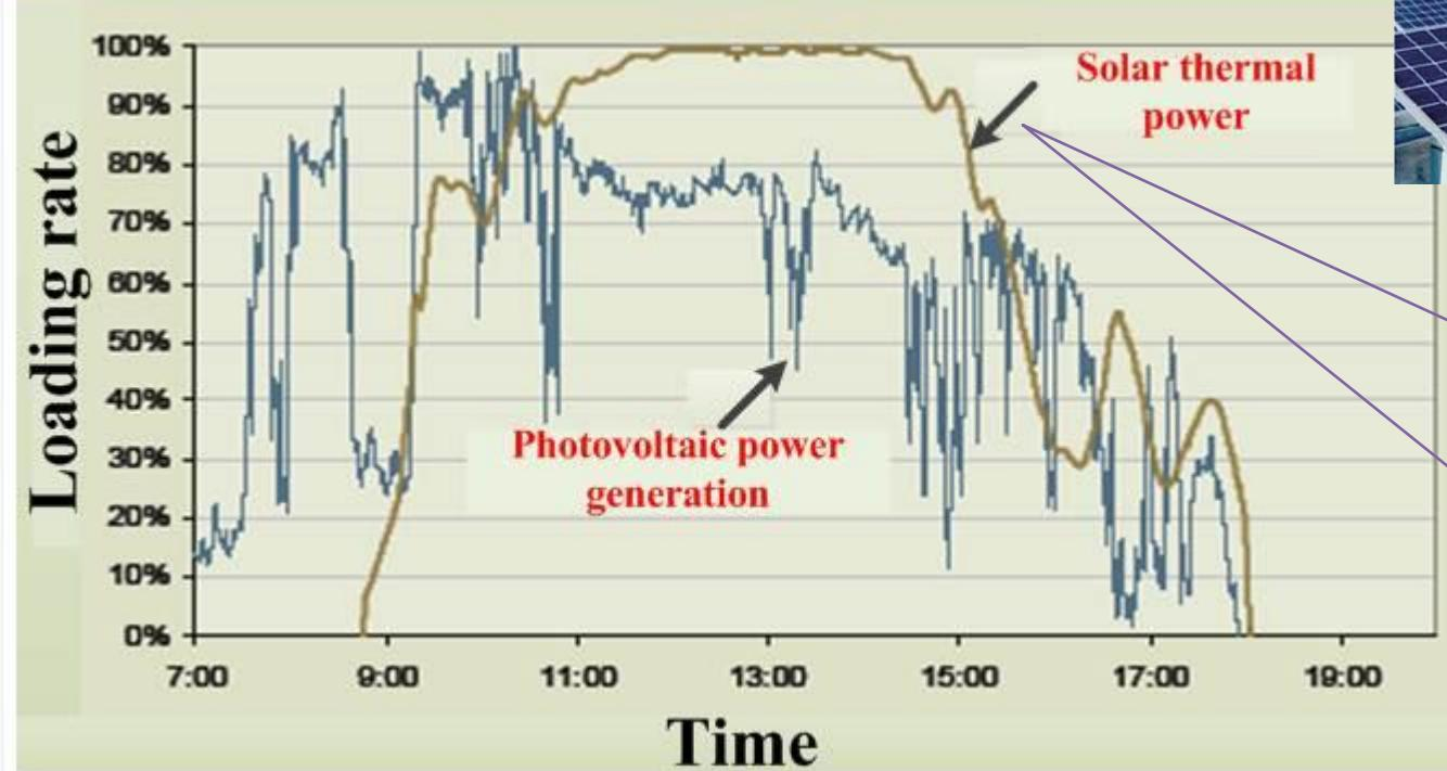
The actual measurement comparison between 50MW thermal power generation and 50MW photovoltaic (California, USA)
