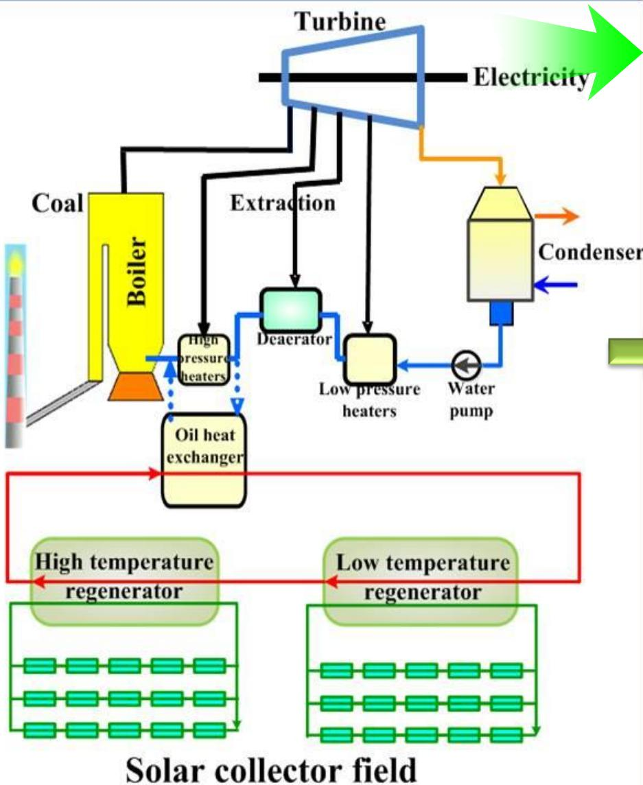
Present: Feed water is heated by extracted steam from turbine
