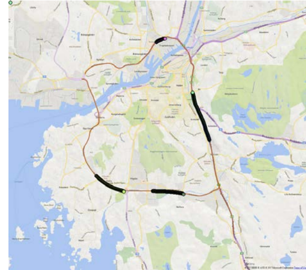
Segments of contiguous ACC operation on the Drive Me test route
