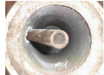
Detailed tuyere with NG Injection Port
