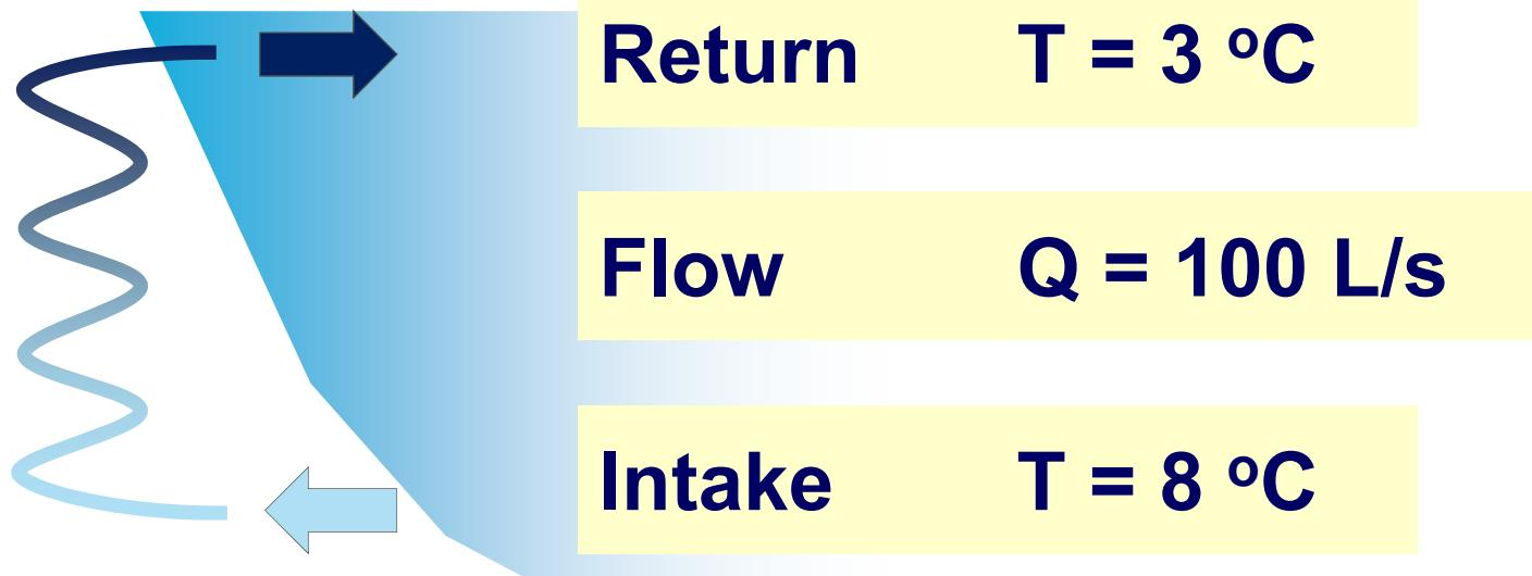
$$\Delta T = 5 \text{ °C} \text{ for } Q = 100 \text{ L/s} \rightarrow \text{Heat} = 2 \text{ MW}$$
