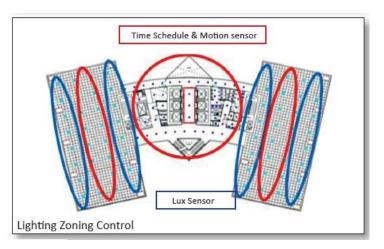
The lighting system was designed by applying zoning system between natural and non-natural lighting.
