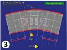
3. Solar path that affects heat gain from solar radiation
