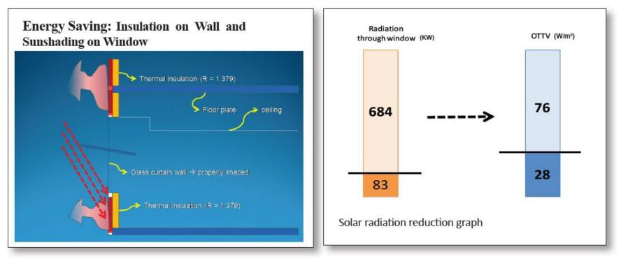
Initial solar radiation through window is 684 kW can be dramatically decreased to 83 kW. It affects to OTTV value which decrease from 76 W/m<sup>2</sup> to 28 W/m<sup>2</sup>. That reduction equal to carbon saving as 1880 ton/year and also equal to CO<sub>2</sub> absorbtion by 165 banyan trees.
