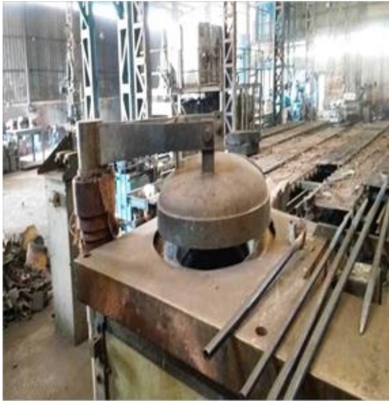
Lid mechanism installed for induction furnace
