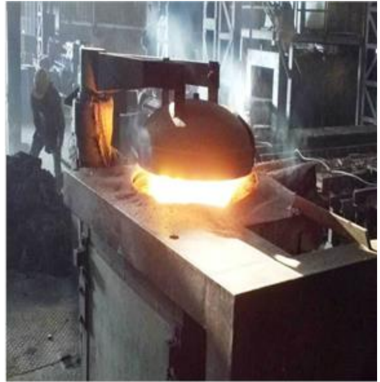
Lid mechanism installed for induction furnace
