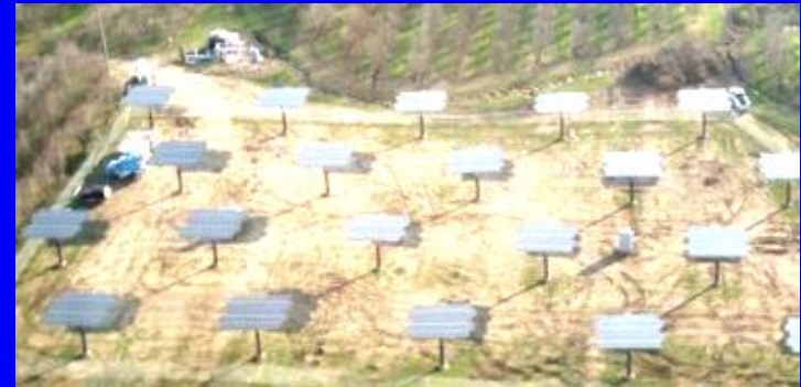
Tracking PV in Almond Grove
