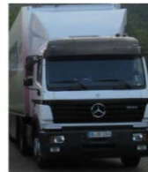
Vehicle 1 from 1996 engine OM 442 LA 436 hp, Euro I
