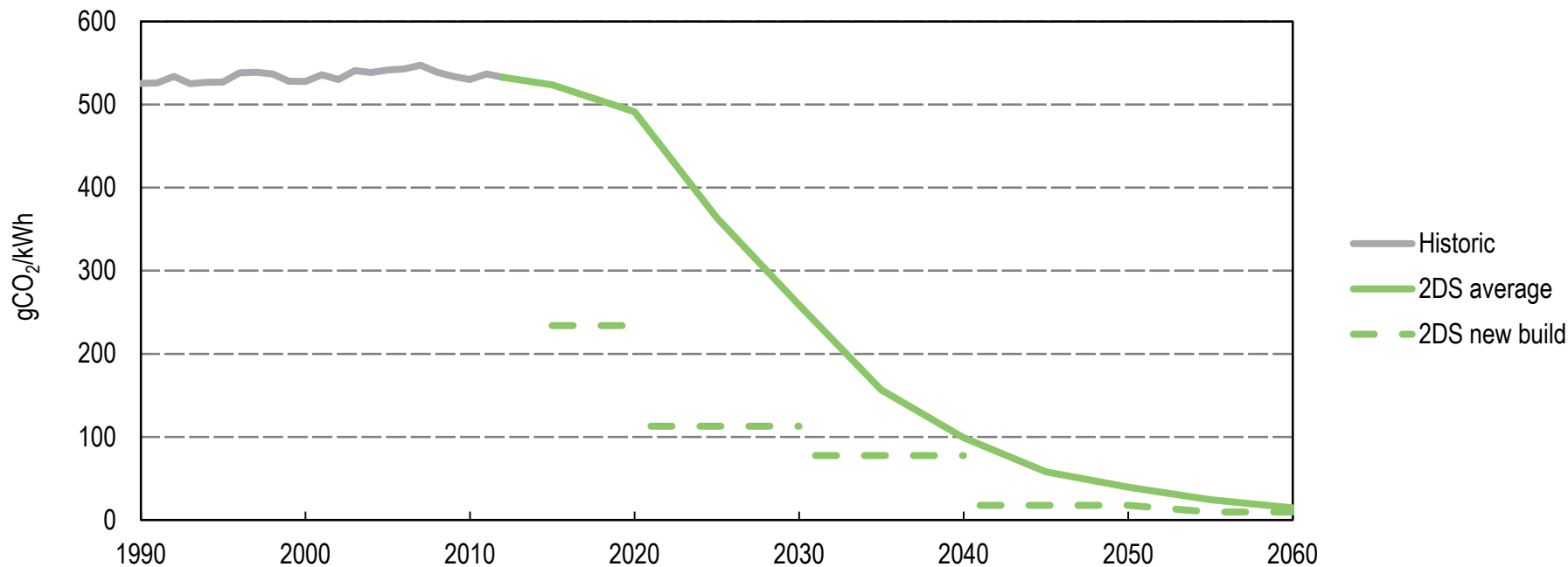
Global fleet average and new-build plants emissions intensity of power generation in IEA scenarios
