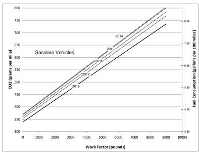
Work Factor = [0.75 x (Payload Capacity + xwd)] + [0.25 x Towing Capacity]
