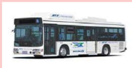
IPS (non-contact recharging) hybrid bus
