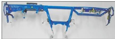
Material: Steel Thickness: 1.0 mm Mass: 8.54 kg
