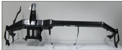
Material: Aluminum Thickness: 1.5 mm Mass: 4.41 kg
