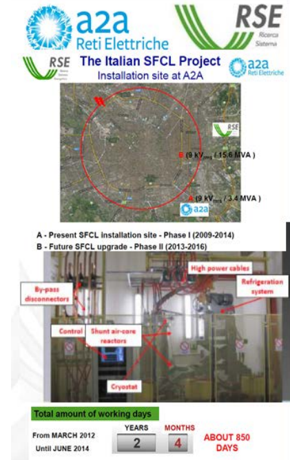
Resistive type, Bi, YBCO 9 kV, 250 A(Bi), 1000A(Y) Bi 2.4years tested in 2014 Y tested in 2016
