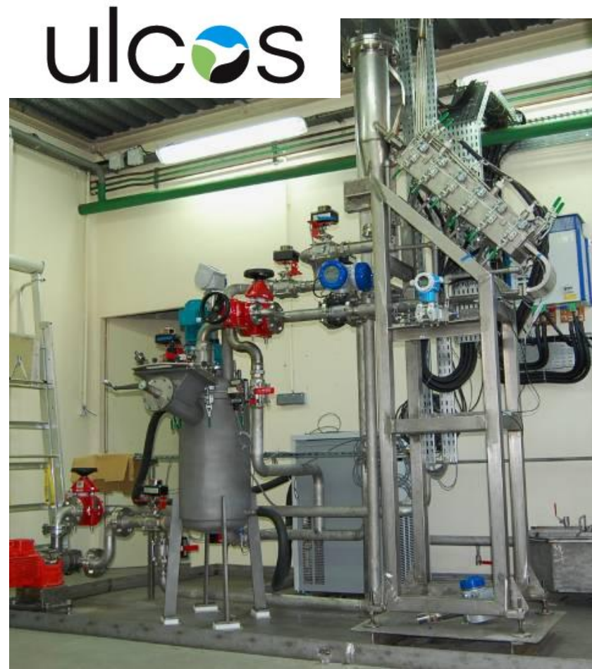
Electrowinning cell demonstrator (ULCOwin, 2011)
