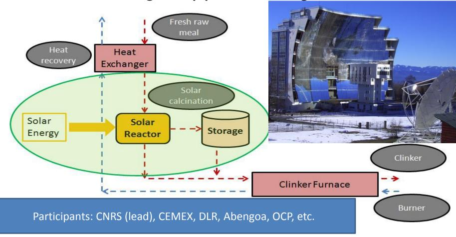
The project aims at developing a 800-1000°C solar process for energy intensive industries such as cement factories, phosphates...
