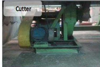
Each Trim blower motor around 10 – 18 KW , modify auto stop when machine not running
