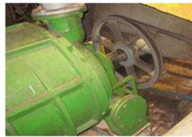
Replace V-belt Nash Pump with Timing Belt will eliminate slippery and reduce electric consumption, PM 3 Done 5 unit
