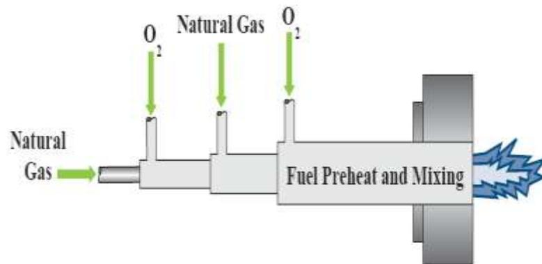
**High Luminosity, Low-NO<sub>x</sub> Burner Design**
