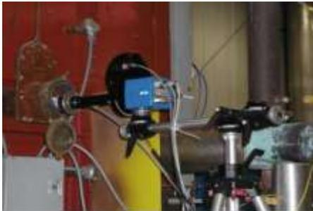
**Bench-Scale Thermal Imaging System Hardware**
