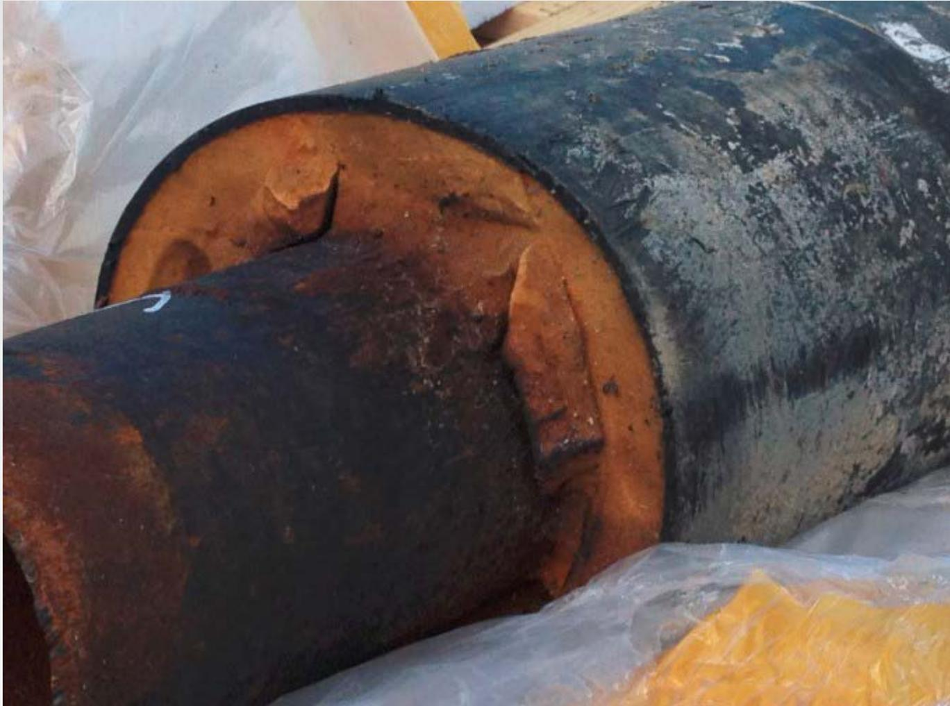
Hypothesis that the degradation of PUR is caused by thermo-oxidation due to oxygen diffusion through PE casing **WAS NOT** confirmed. The shear strength decreases fast at the beginning and then reaches a constant value which depends on temperature but not time.
