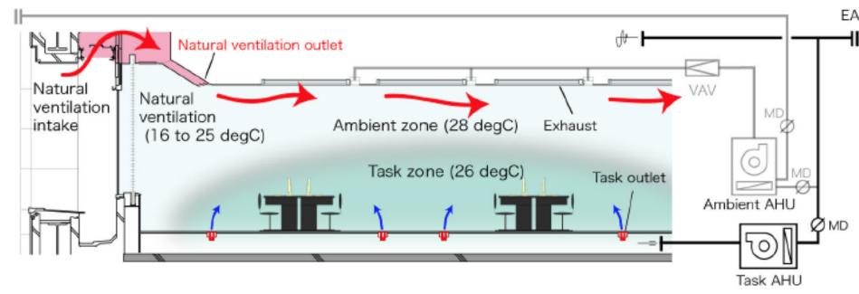
SPRING AND FALL, AMBIENT ZONE IS NATURALLY VENTILATED IF POSSIBLE (CONDITIONS ARE PRESSURE DIFFERENCE, OUTSIDE AIR TEMPERATURE, HUMIDITY AND ENTHALPY).
