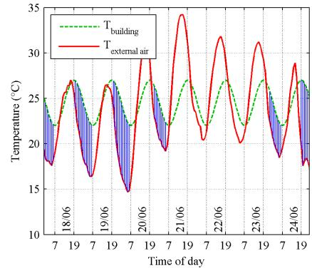
Shaded areas show the climatic cooling potential during one exceptionally hot week in summer 2003 for Zurich SMA (ANETZ data)
