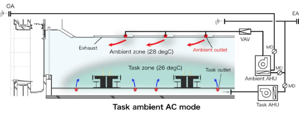
IN SUMMER TIME, TASK AND AMBIENT ZONE IS ACHIEVED BY UNDER FLOOR AIR SUPPLY (FOR TASK ZONE) AND CEILING OUTLET (FOR AMBIENT ZONE)
