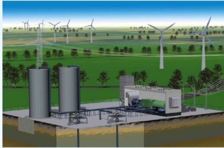
ADELE – ADIABATIC COMPRESSED-AIR ENERGY STORAGE FOR ELECTRICITY SUPPLY
