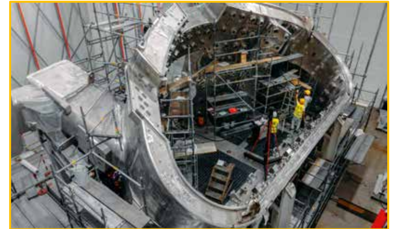
5 Vacuum Vessel sectors on-site, the others in advanced stages of production
