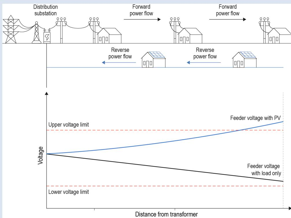
Source: Kwang-Hoon Yoon et al. (2022). [Operation Method of On-Load Tap Changer on Main Transformer Considering Reverse Power Flow in Distribution System Connected with High Penetration on Photovoltaic System](#), as modified by the IEA.
