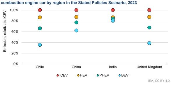
Life cycle emissions of a medium-sized car by powertrain relative to a gasoline internal
