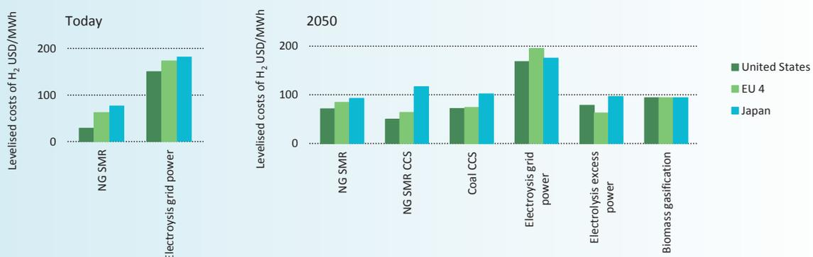
**KEY POINT:** Hydrogen produced from grid electricity is costly compared to alternative generation pathways. For cost-effective renewable hydrogen, the availability of low-cost, surplus renewable electricity is a prerequisite. \*\*\*\*\*
