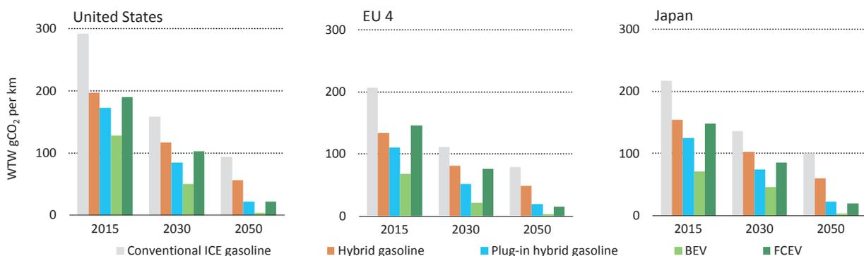
Note: Stock on-road WTW emissions include the upstream emissions from liquid fuel production as well as power and hydrogen generation. The fuel economy of the vehicle stock is based on the fuel economy of new vehicles sold, assumptions on average age and a gap factor of approximately 20%, accounting for the difference between test-cycle fuel economy and on-road fuel economy.
