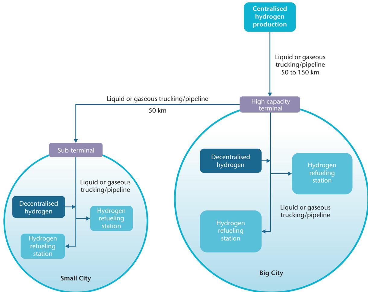
**KEY POINT:** Different hydrogen generation, T&D and retail pathways will develop over time. In the underlying model scenario, the centralised supply of small cities happens via terminals based in large urban areas.
