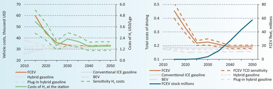
**KEY POINT:** While FCEV costs drop rapidly as sales ramp up, the cost of hydrogen at the pump drops much more slowly. Hydrogen costs decline quickly as long as stations are clustered around early demand centres. When the hydrogen refuelling network is expanded to provide the coverage necessary to sell millions of FCEVs, hydrogen costs see another increase.
