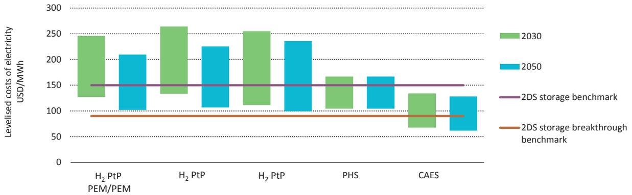
**KEY POINT: Hydrogen-based storage technologies can be competitive at low electricity input prices.**
