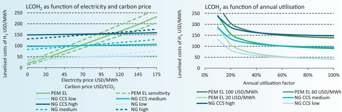
Notes: PEM EL = proton exchange membrane electrolyser; LCOE = levelised cost of energy; NG = natural gas; for the left-hand graph, annual loads of 85% are assumed for all technology options, and the dashed line marks the sensitivity of LCOE for hydrogen from a PEM electrolyser with a 30% variation in cost and a 10% variation in efficiency.
