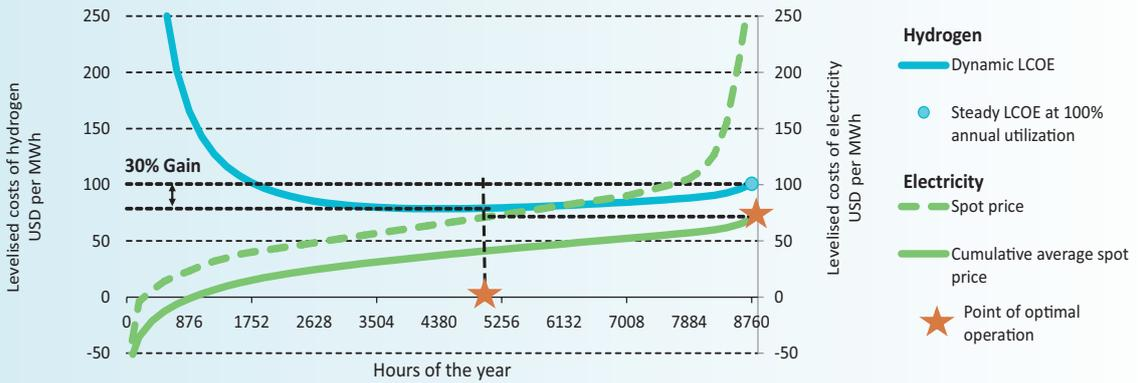
**KEY POINT:** A more dynamic use of the electrolyser with optimised operation with respect to input electricity costs and annual utilisation rate can significantly reduce LCOE of hydrogen generation.
