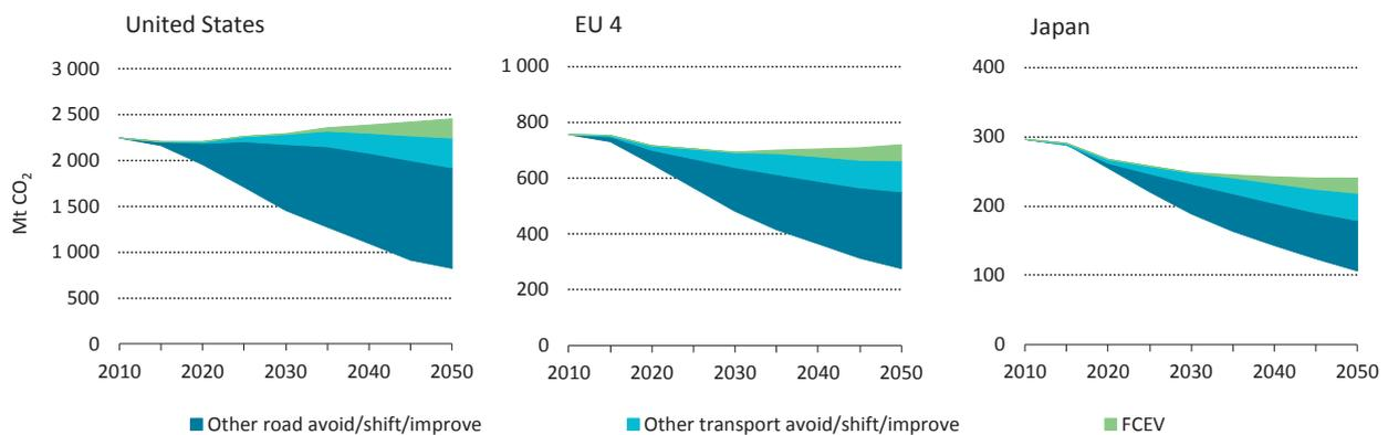
**KEY POINT:** By 2050, the large-scale deployment of FCEVs in the transport sector could account for 14% of the annual carbon mitigation reductions necessary to switch from a 6DS to a 2DS emission trajectory.
