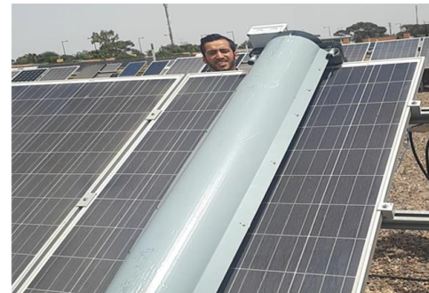
PV-C ROBOT Solar panel cleaning robot
