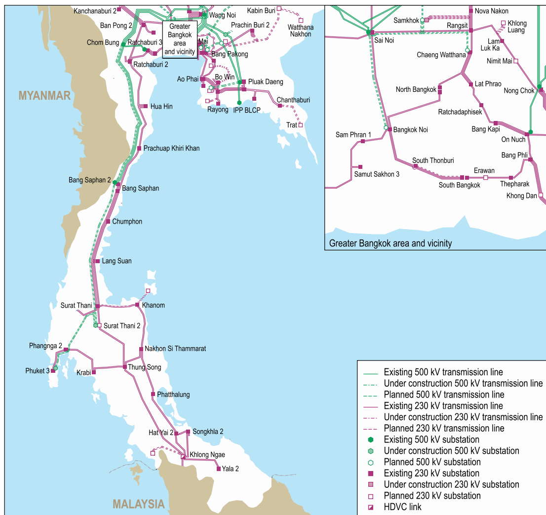
Figure 2.5 • Detailed schematic of Thailand's transmission network in the southern region
