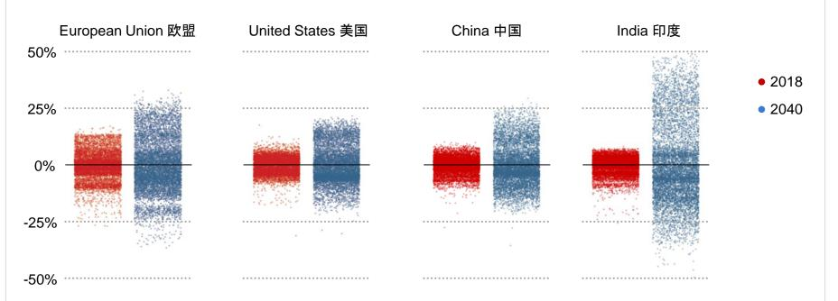
Flexibility requirements in China is expected to double by 2040. A wide set of distributed flexibility sources, including storage and demand-response will be needed to ensure electricity security
