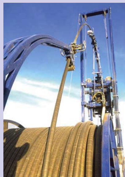
Figure 2.14 • Coiled tubing unit
