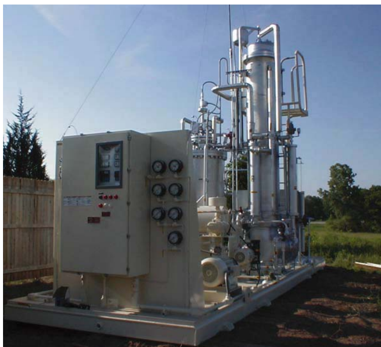
Figure 5.5 • Prototype small-scale GTL plant
