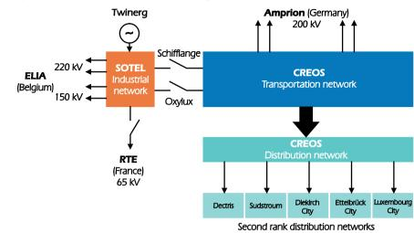
Figure 5.5 Electricity network structure in Luxembourg, 2013
