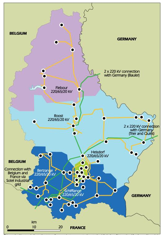
Figure 5.6 The electricity grid of Luxembourg, 2014
