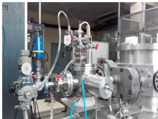
Experimental set-up for the study of tritium permeation barriers (Source: CIEMAT, Spain)
