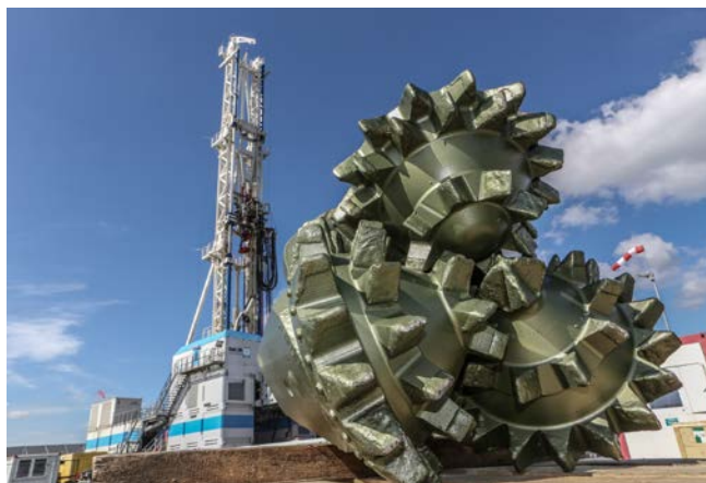
Rotary drilling bit in front of a drilling rig. (Source: Stadtwerke München SWM)
