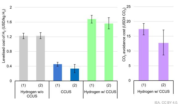
Levelised cost of hydrogen production and CO<sub>2</sub> avoidance cost under Scenarios 1 and 2
