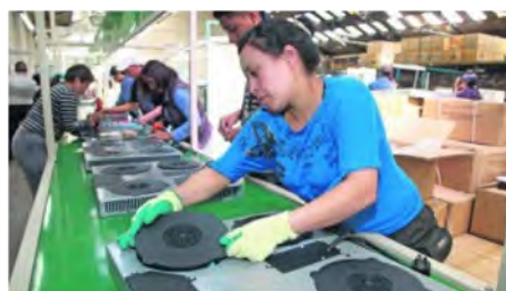
An electric induction cooktop being assembled at Cuenca's Inudrama factory.
