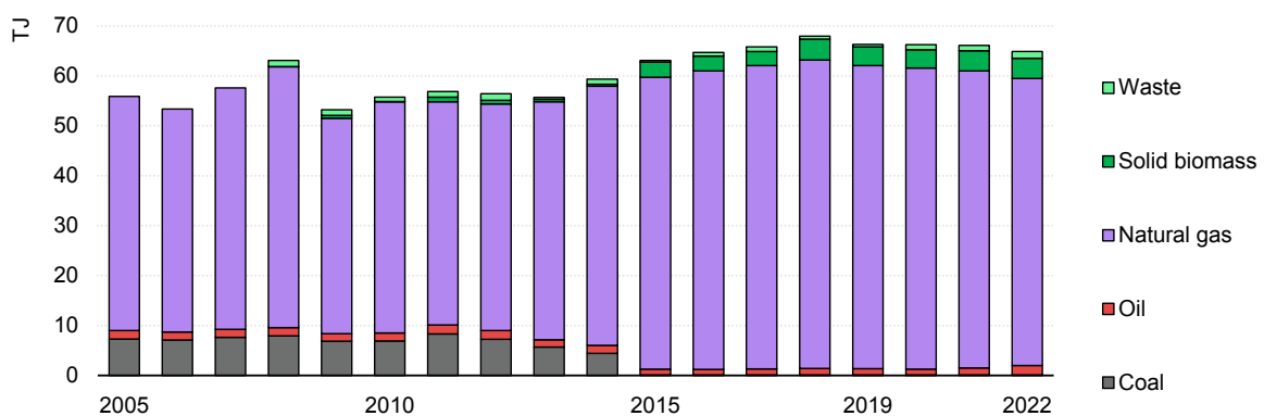
Figure 3.3 District heating supply by source and carbon intensity in the United Kingdom, 2005-2022
