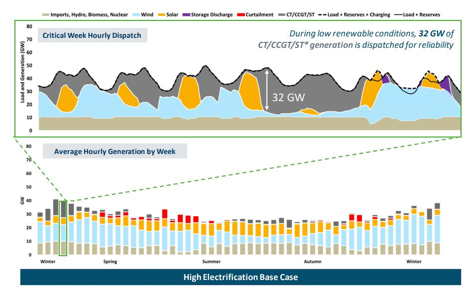
\* Could represent natural gas, hydrogen, or other zero-carbon fuel blend burned in CT/CCGT, or dispatchable long-duration storage if viable technology emerges. More generally, this could represent any firm capacity, e.g. nuclear SMRs and Gas with CCS could also play this role.
