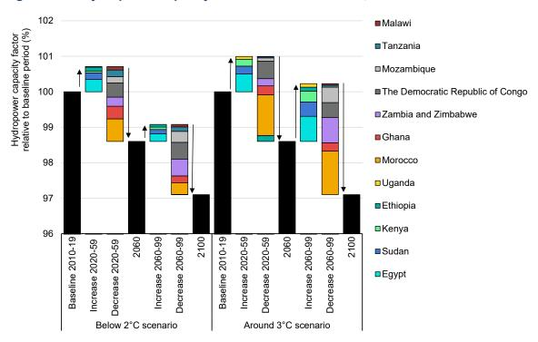
Figure 3.30 Hydropower capacity factor evolution in Africa, 2020-2099
