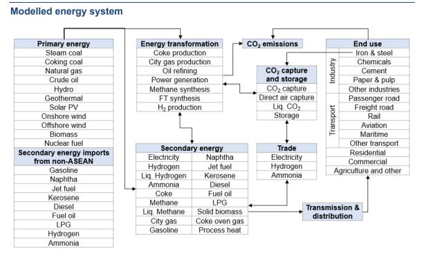
Notes:  $CO_2$  = carbon dioxide,  $H_2$  = hydrogen, FT = Fischer-Tropsch, liq. = liquid, LPG = liquefied petroleum gas, PV = photovoltaic.
