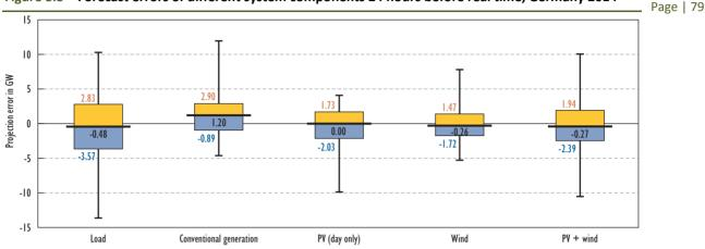
Figure 3.3 • Forecast errors of different system components 24 hours before real time, Germany 2014
