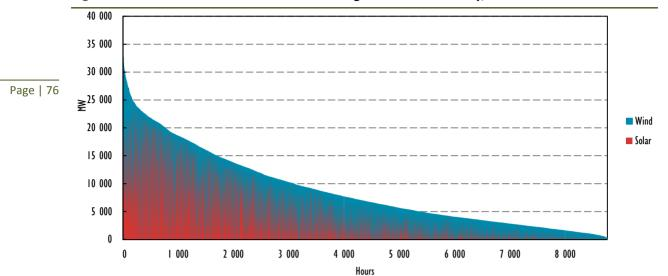
Figure 3.1 • Load duration curve of wind and solar generation in Germany, 2013
