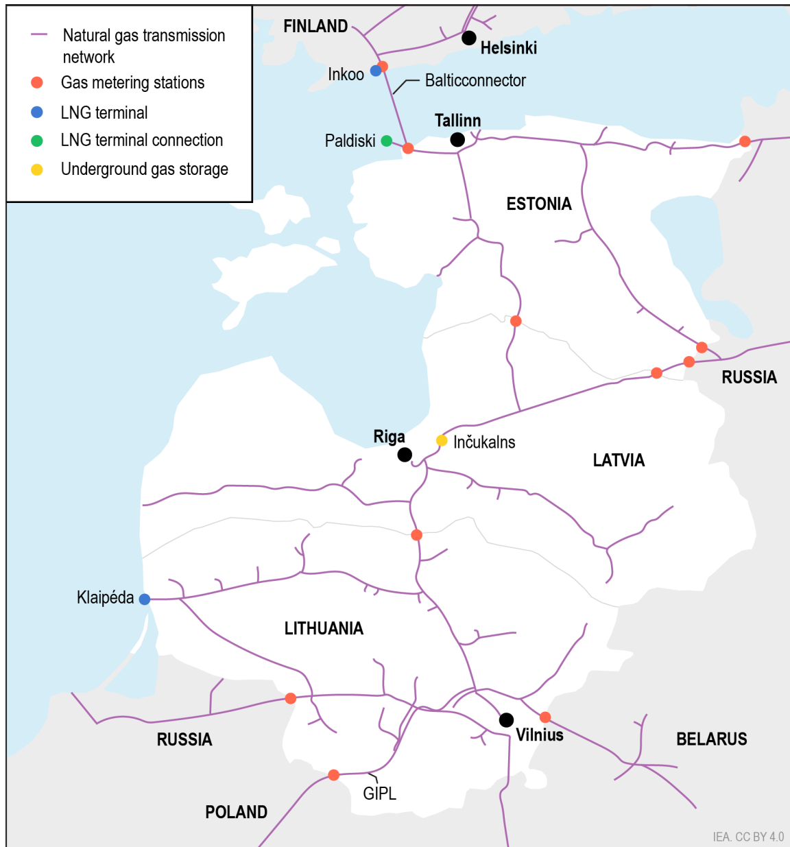
Figure 7.3 Baltic natural gas transmission network
