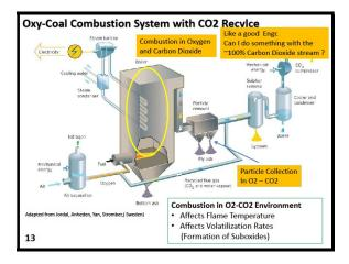
He provided an overview of how stage pressurized oxy-combustion technology can be used to increase efficiency and to lower capital and operating costs. Design estimations with Powder River Basin coal indicate a 5% improvement in efficiency over conventional oxy-combustion technology.
