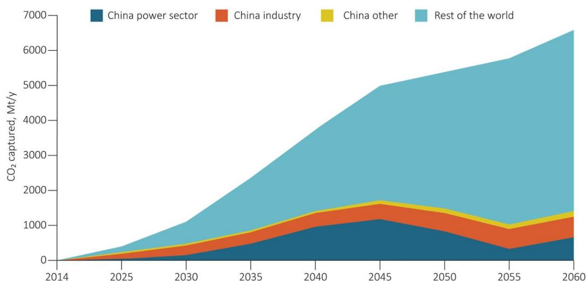
Figure 1 The contribution of CCS in China's power and industrial sectors to total CO<sub>2</sub> captured in the IEA's 2DS to 2060 (IEA, 2017a)
