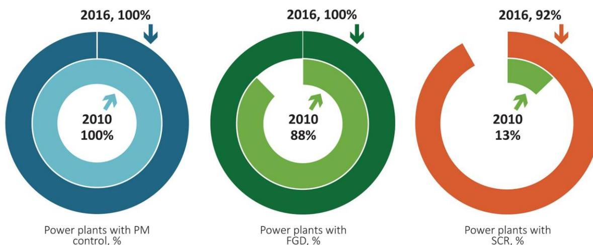
Figure 8 Installation rates of pollutant control devices in China's utility coal fleet in 2010 and 2016 (Li, 2017a)
