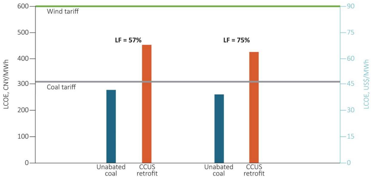
Figure 20 LCOE for unabated coal plant and CCS retrofits at different load factors, showing average coal tariffs (China Energy unit average for 2018) and wind power tariffs (Huaneng wind fleet average for 2017) for comparison
