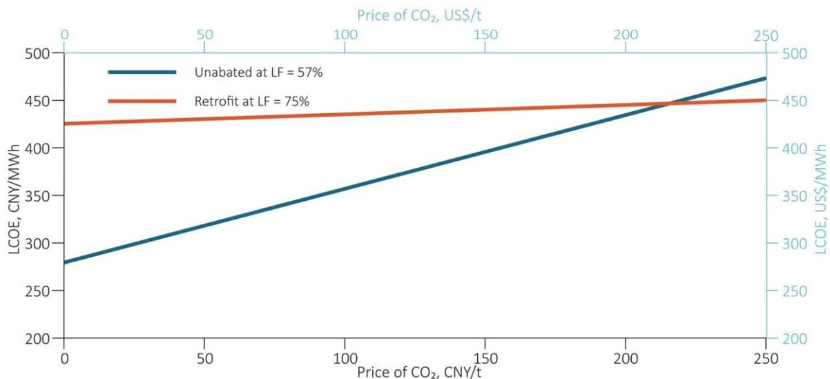
Figure 23 The effect of increasing CO<sub>2</sub> price on the LCOE of unabated and retrofitted coal plants
