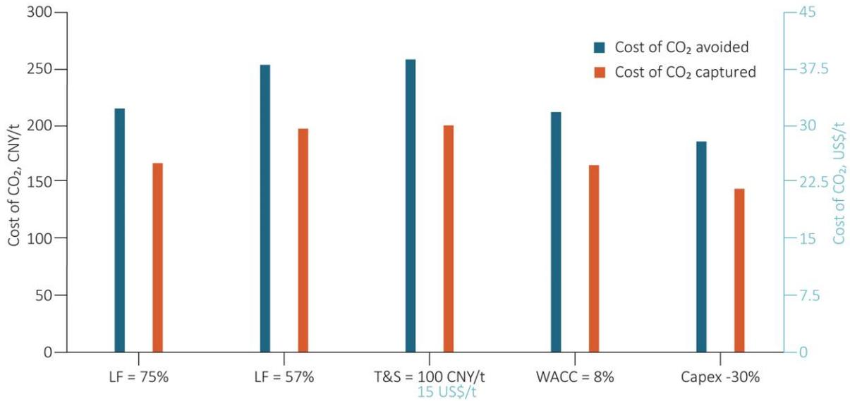
Figure 25 The cost of CO<sub>2</sub> avoided and captured for various CCUS retrofit cases in 2025
