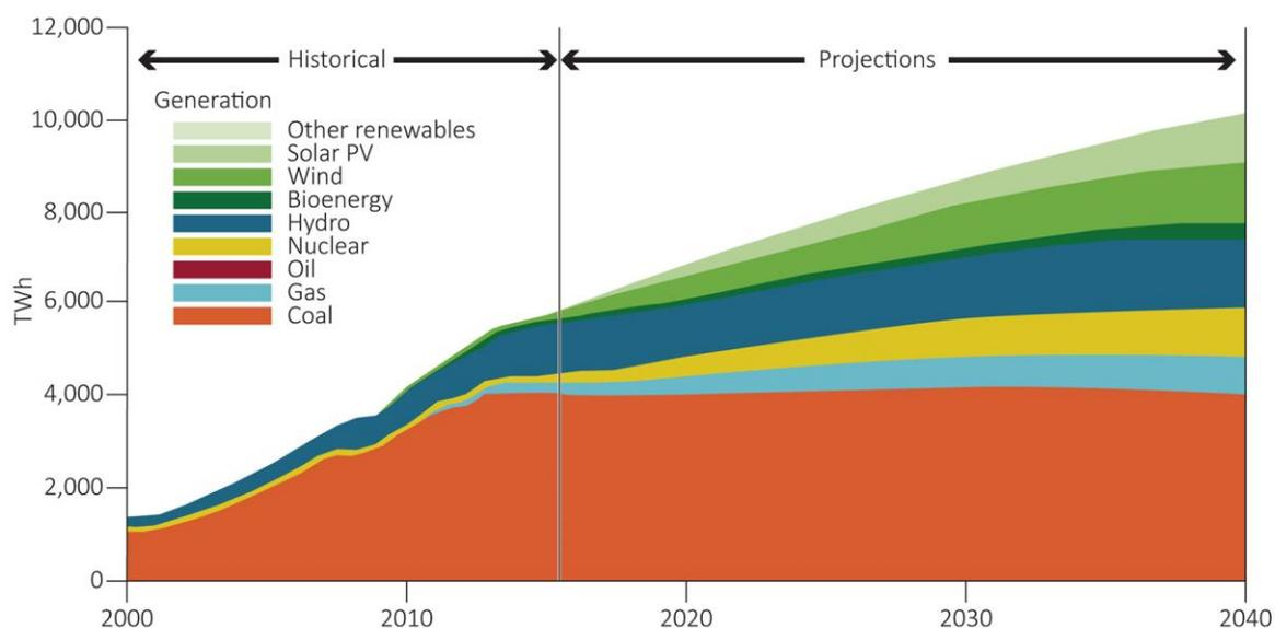
Figure 4 Historical and projected changes in China's power generation mix under the IEA's 'New Policies Scenario' (IEA, 2017a)
