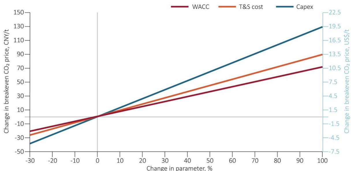
Figure 17 The effect of varying weighted average cost of capital (WACC), capture plant capex, and transport and storage cost on the CO<sub>2</sub> price required for the retrofit project to break even
