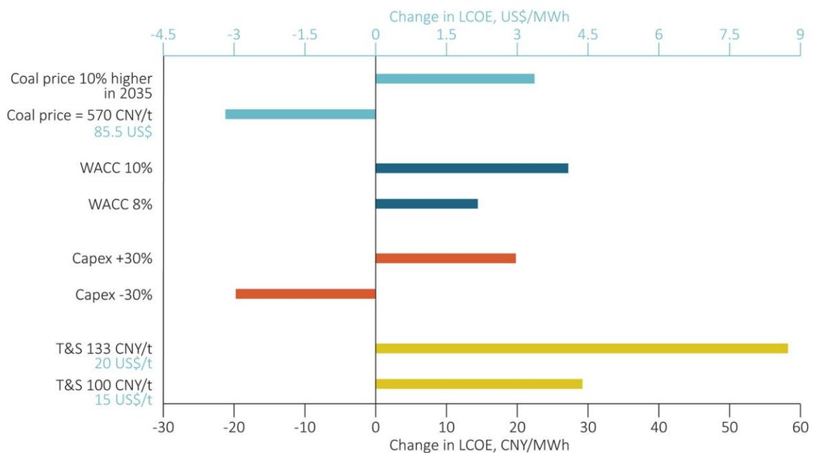
Figure 24 The effect of changes in coal price, weighted average cost of capital (WACC), capture plant capex, and transport and storage (T&S) cost on LCOE
