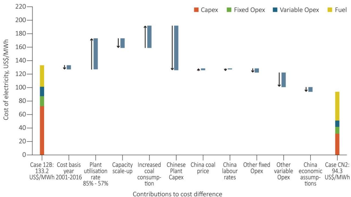
Figure 11 The difference in first year cost of electricity between the NETL baseline (new-build, Case 12B) case for a supercritical coal power plant with post-combustion capture and an equivalent retrofit case in China (Case CN2), showing the contributing factors (Singh and others, 2018)
