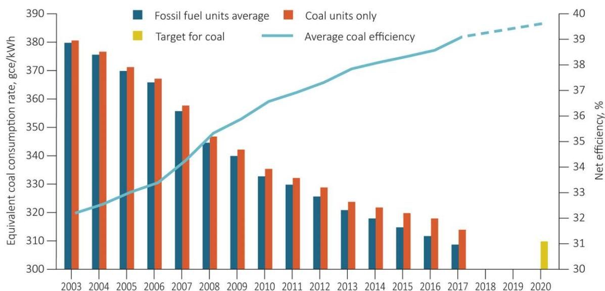
Figure 7 The reduction in average equivalent coal consumption for all fossil-fired units (including gas-fired plant) since 2003. Estimated from these figures are the approximate average coal consumption for coal units alone and the corresponding average efficiencies. The 2020 target for coal units is also shown (Li, 2017, 2018a)
