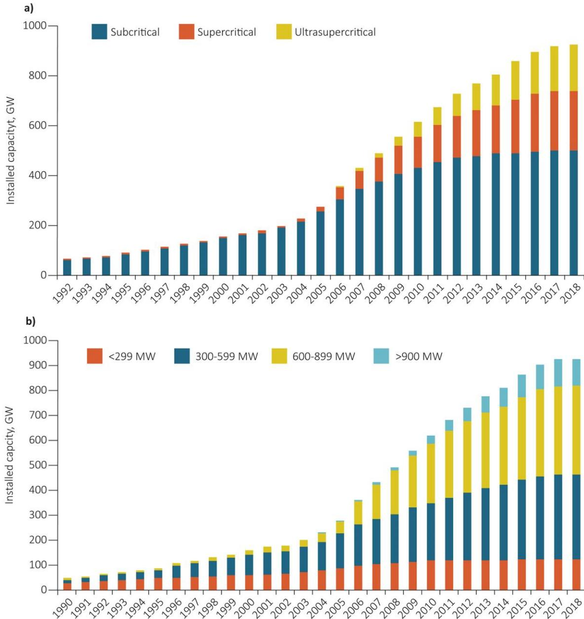
Figure 6 The composition of China’s current coal power fleet by unit commissioning year, showing a) steam type and b) unit size (Platts, 2018)
