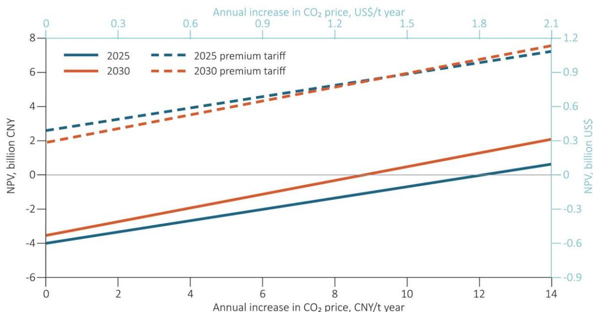
Figure 19 The variation in NPV of retrofit projects for different linear growth rates in CO<sub>2</sub> price, shown for investment in 2025 and 2030 (baseline parameters) and with a premium CCUS tariff of 40% above the unabated coal tariff
