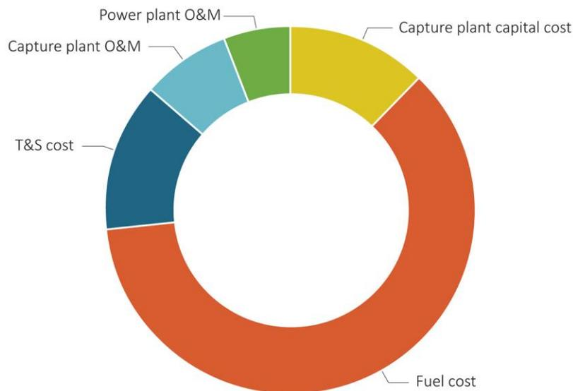
Figure 21 The breakdown of cost contributions to the LCOE for the baseline retrofit case
