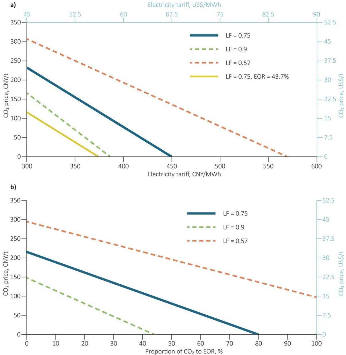
Figure 16 a) Combinations of CO<sub>2</sub> price and electricity price at which retrofit projects can break even, shown for different load factors and an EOR scenario which breaks even under baseline conditions. b) Combinations of CO<sub>2</sub> price and EOR sales at which retrofit projects break even, shown for different load factors
