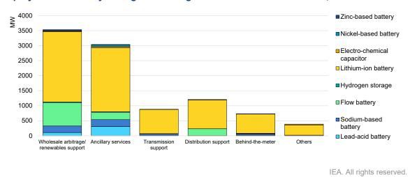
Deployment of battery storage technologies in different value streams, 1987-2020
