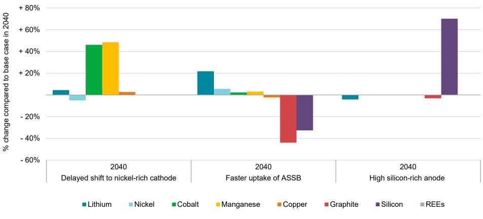
Change in mineral use for EVs in alternative cases relative to the base case in the SDS
