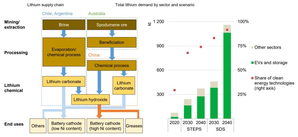
Note: Some spodumene ore is directly consumed for ceramic material.
