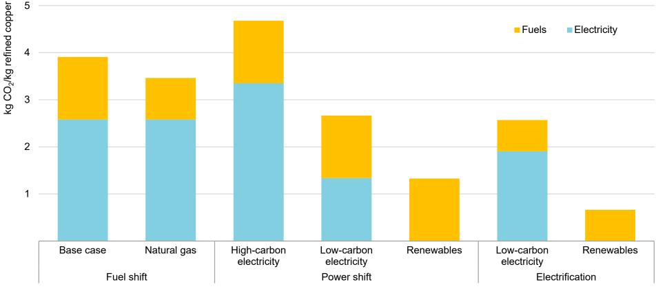
Energy-related CO<sub>2</sub> emissions intensity for an indicative refined copper production project under different energy consumption scenarios
