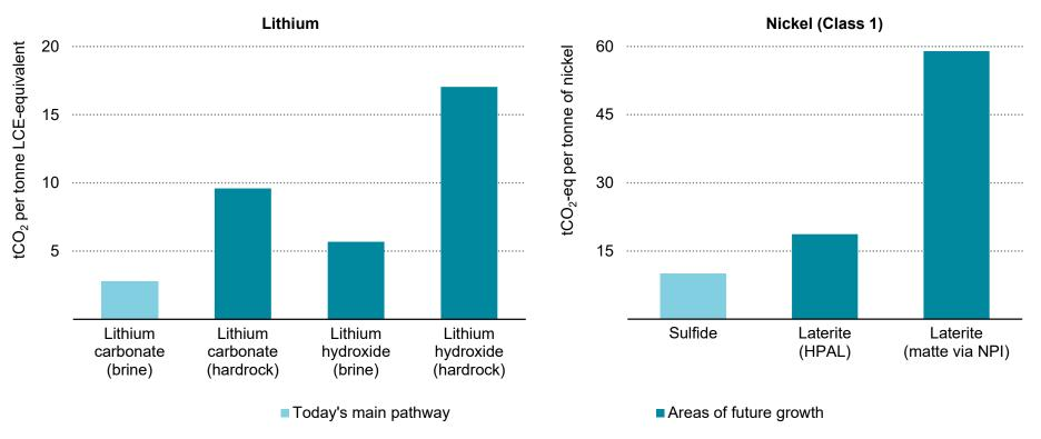
GHG emissions intensity for lithium and nickel by resource type and processing route
