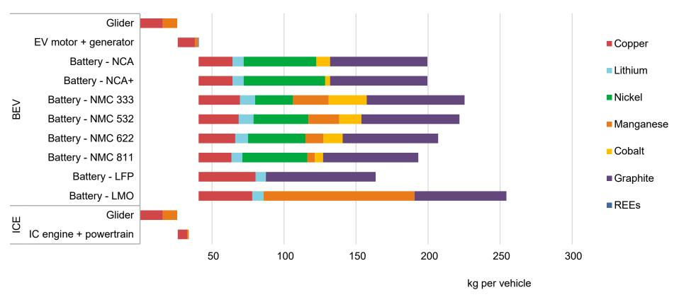
Typical use of minerals in an internal combustion engine vehicle and a battery electric vehicle
