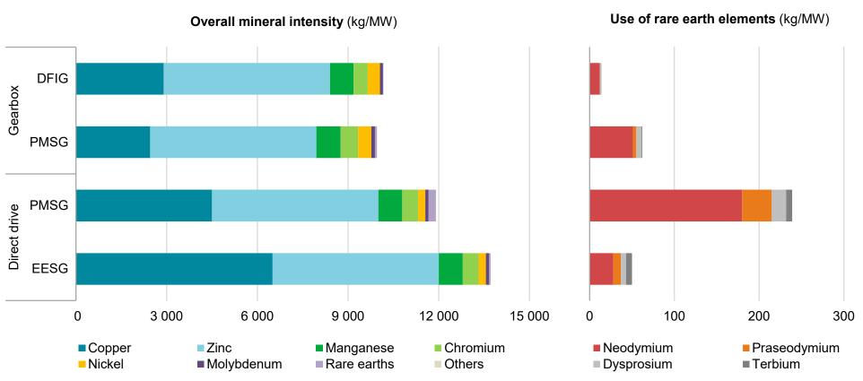
Mineral intensity for wind power by turbine type
