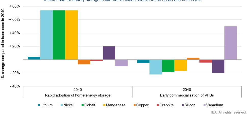
Mineral use for battery storage in alternative cases relative to the base case in the SDS
