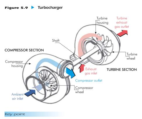
Turbochargers recuperate energy from exhaust gases to improve engine efficiency.
